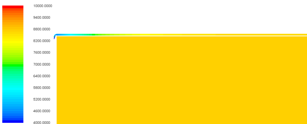
Figure 12: CFD-simulation results: pressure distribution [Pa] in the upper part of the FFG element and the outflow spacer
