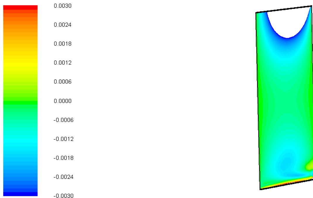
Figure 8: CFD-simulation results: horizontal velocity components [m/s] in the fluid chamber with labyrinth spacer
