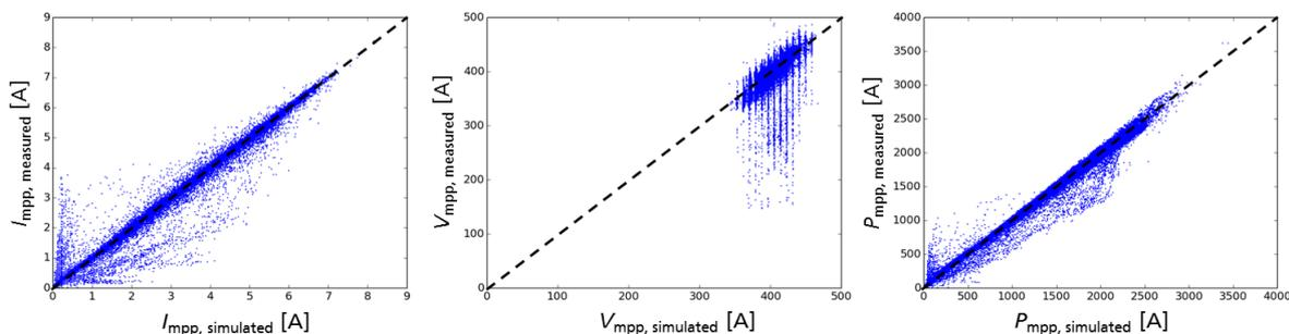
Figure 5: Comparison of simulated and measured DC-output of one string of BIPV system B.
