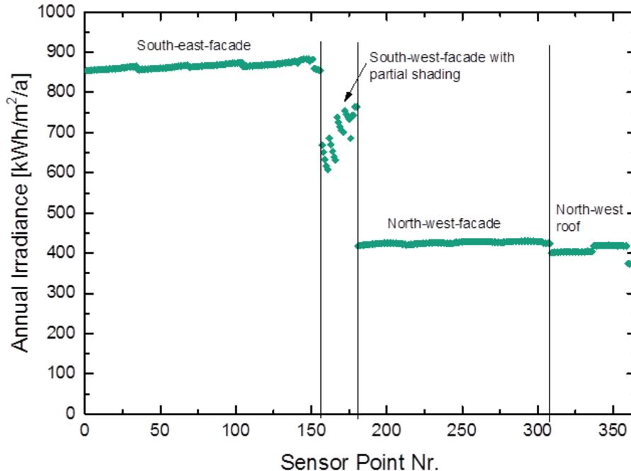
Figure 3: Example result for the irradiance calculation via ray-tracing in step 1. For various sensor points on the building skin (where PV-cells could be applied), the irradiance values integrated over a whole year have been calculated. Based on such a calculations, it can be decided where BIPV is a good solution. Also partial shading effects due to neighbouring buildings are included.
