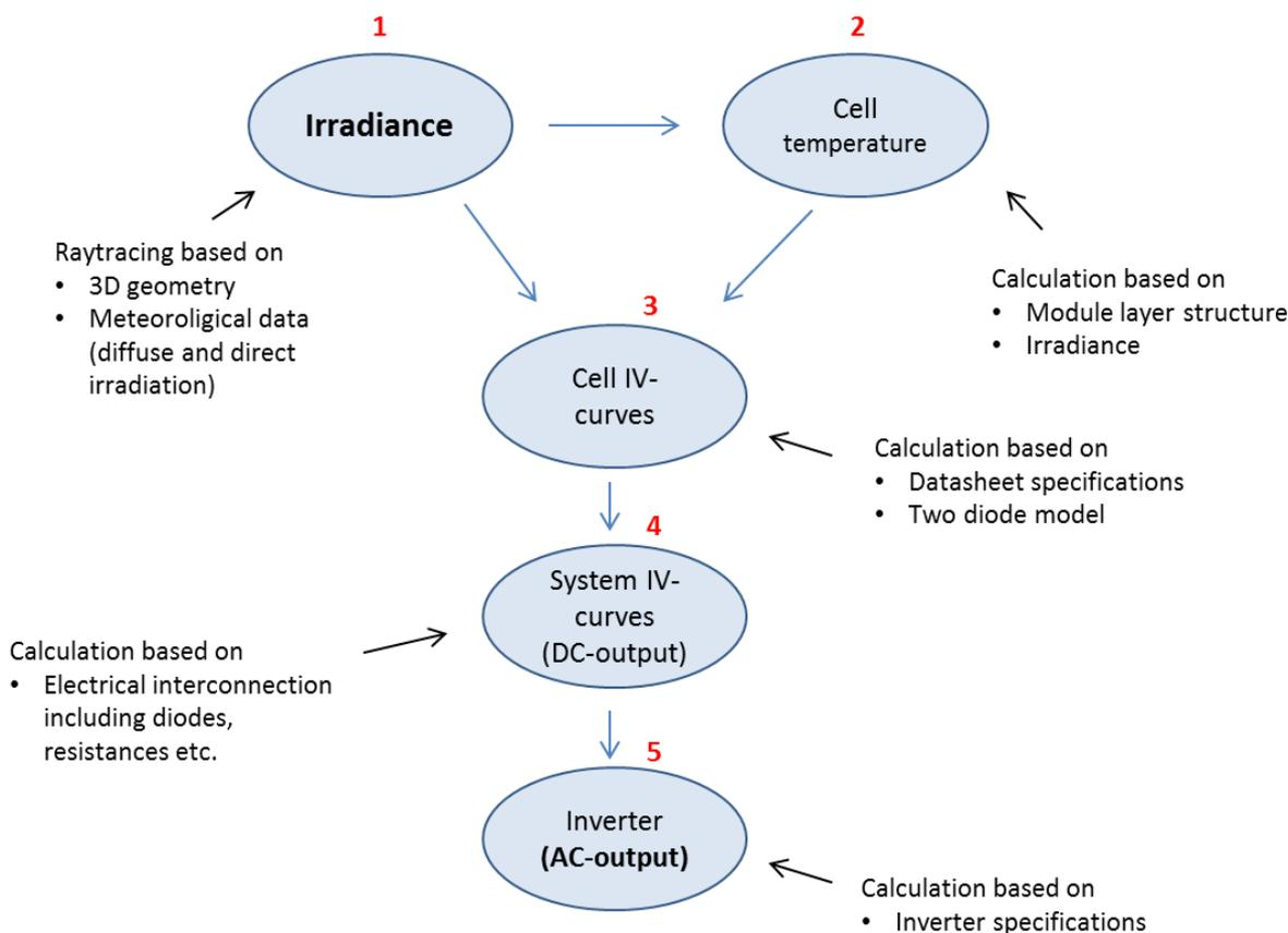
Figure 1: The BIPV simulation tool chain. Starting from the building and BIPV system geometry and meteorological data, the time dependent electrical yield of the system is calculated.
