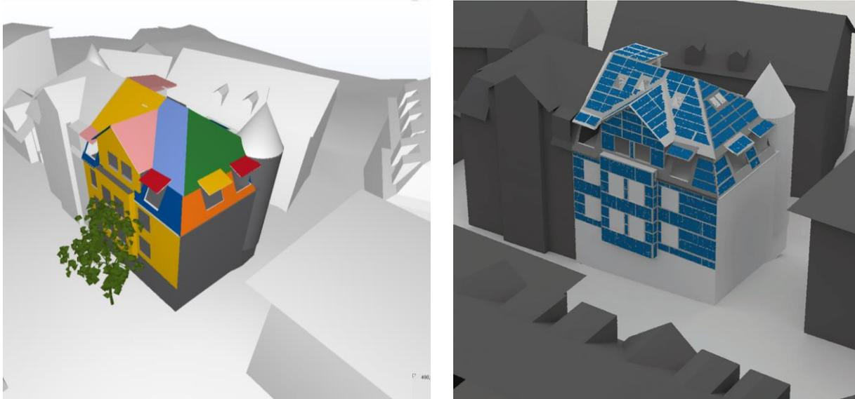
Figure 2: Example for the geometry translation from IFC to Radiance. On the left a visualization of the architectural IFC file (with Solibri, with pseudo-colors due to wrong material definitions). On the right the translated and post-processed Radiance file (visualized with rshow). The radiance file has been processed after the translation: Removal of tree, adding PV-panels, adjusting material properties for ray-tracing.
