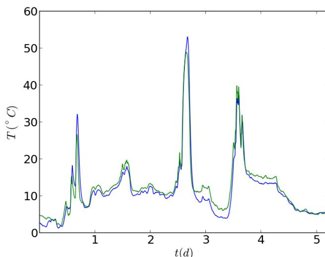
*Figure 4: Temperature simulation (blue line) compared to measured temperature (green line) at 5 days. High irradiance on day 3 leads to high module temperatures. This is relevant to the module performance but also for temperature simulation of the building.*
