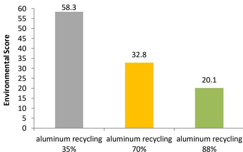
Figure 3 Environmental Score of the façade system based on aluminum from different scenarios for aluminum recycling rate (ReCiPe 2008). One point on the single-score-scale represents the average yearly environmental impact of one European citizen.
