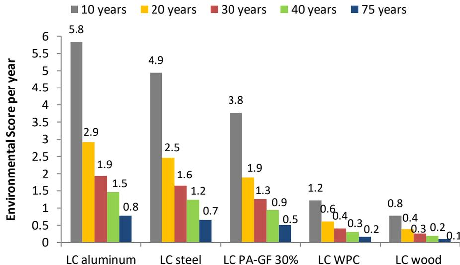
Figure 2 Environmental Score of five different Façade-Frame-Systems (ReCiPe 2008). One point on the single-score-scale represents the average yearly environmental impact of one European citizen. The comparison shows the environmental impact of a façade-system based on aluminium, steel, glass-fiber reinforced polyamide (PA-GF 30%), wood-plastic-composite and wood. LC=Life Cycle.
