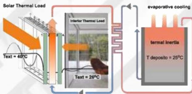
Principle of Fluid Flow Glazing as actively controllable radiant cooling and heating element
