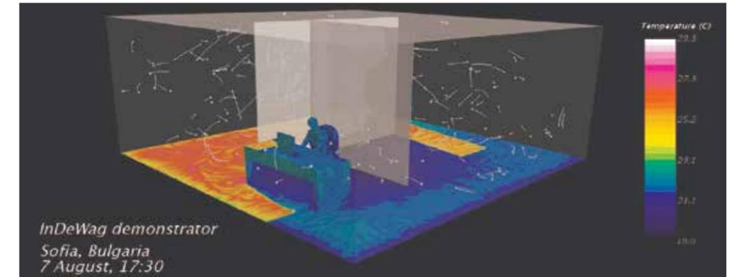
Fig. 8 Temperatures and air movements in the demonstrator pavilion resulting from CFD simulation.
