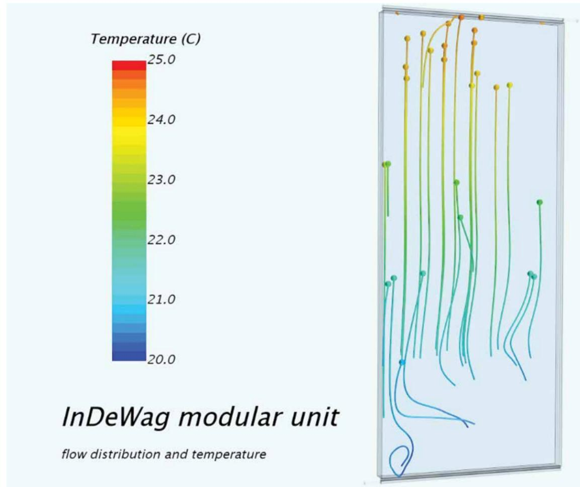
Graphical representation of computational fluid dynamics (CFD) results of the water flow glazing unit.
